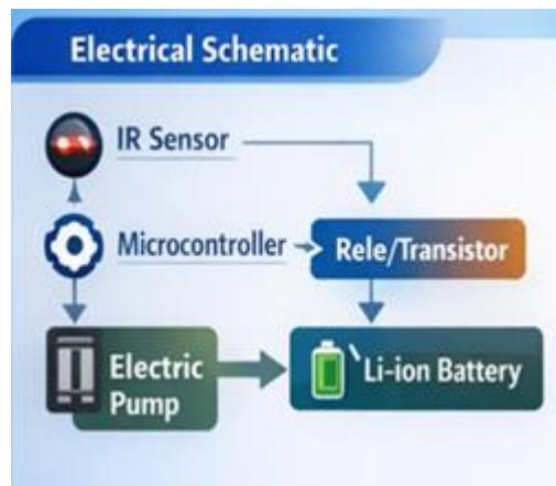
The control signal is used to turn on and off an electric pump through a relay or transistor. Electrical and functional diagrams were created, and automatic and manual control modes of the device were tested. During the study, the stability of the device's operation, response speed, and energy consumption were evaluated.
