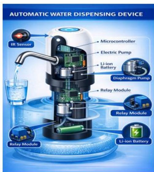
**Methodology.** This study is aimed at developing and analyzing an automatic water dispenser, using a systematic and practical approach. Initially, the literature on sensor and automatic control systems was studied, and a device model based on an infrared sensor and a microcontroller was developed. The principle of operation of the device is based on detecting user movement using an IR sensor and processing this signal using a microcontroller.
