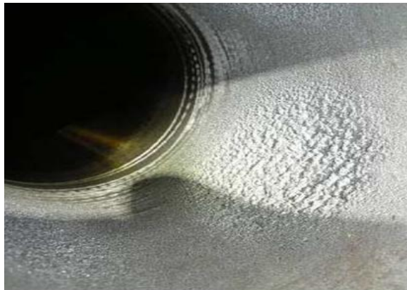
Figure 5. Erosion damage due to cavitation on the throat surface of a multi-nozzle oil jet pump (Zhang et al., 2014)
