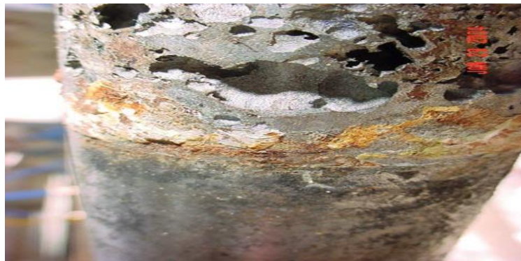
Figure 8. The characteristic smooth scalloping and fine porosity indicative of a stray current corrosion in stainless steel
